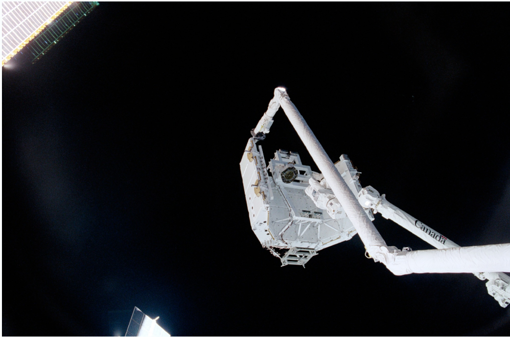
Figure 6) Transfer of the transport pallet from Canadarm2 to the Shuttle Canadarm, known as the Canadian handshake. Credit: NASA, image STS100-347-007. Public domain.
